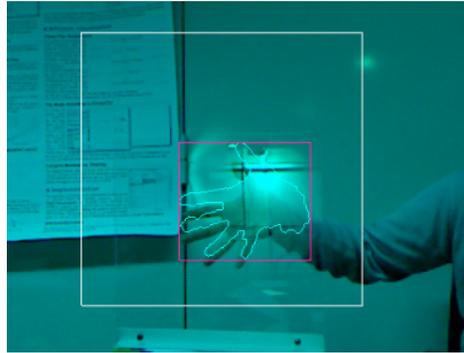
Figure 6: Tracking of the hand using Kinect.
